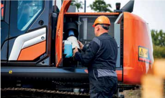
Access to filters has improved on the ZX135US-7B.
