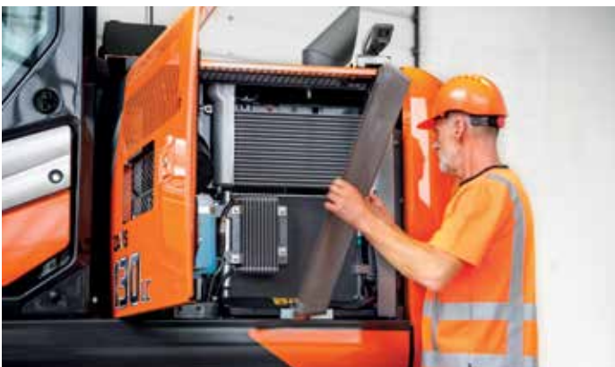
Enlarged radiator door (ZX130-7B) provides easy access for cleaning and maintenance.
